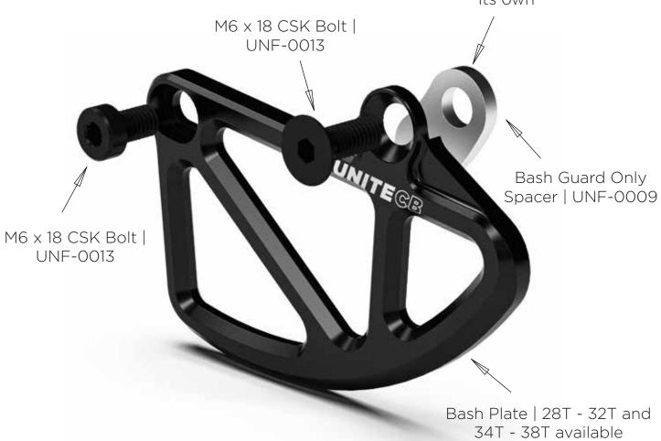
Please ensure ICSG-05 mounts are clean before mounting the guard to the frame. Torque both bolts to a minimum of 6 N/M
