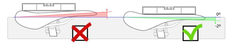
The saddle must be positioned horizontally or at an angle not less than -2 °. Must be considered the central area which mainly supports the rider.
