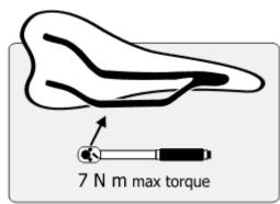
The aproppiate torque depends on the type of fixation used, as a general rule should be tightened enough so that the seat is held firmly and do not move. Although the rails are solid and very resistant, is recommended not exceed 7 Nm (Newton meter).
