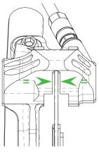
NOTE: We do not recommend pumping the lever to push pads out to align caliper at this point. See the next section regarding the alignment of pistons.
