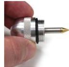
**4** IF THERE'S a puncture object, like nail or screw, note its angle when removing from tread and insert in the path.
