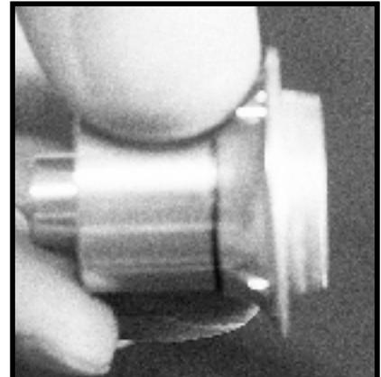
Figure 10 - adjusting cone
