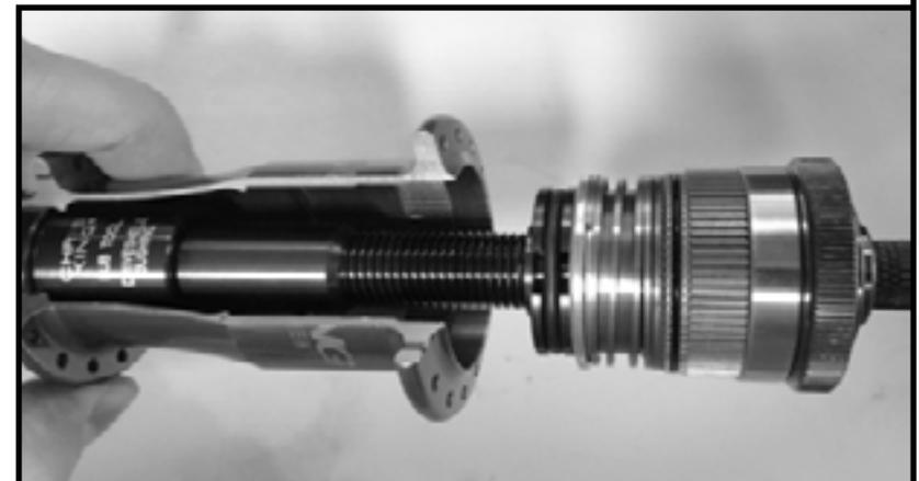
Figure 45 - remove RingDrive™ assembly
