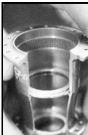
Figure 55 - spring retainer
