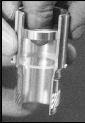
Figure 61 - drive shell seal & bearing
