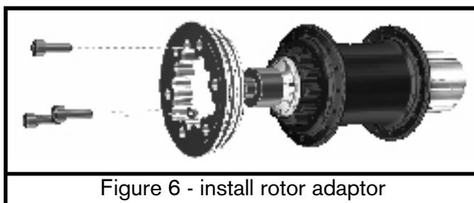
Figure 6 - install rotor adaptor
