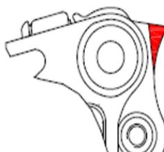
Figure 48: correct position of the links to insert the lever
