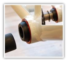
Insert the right side adapter into BB30 or PF30 Bottom bracket by hand. Note: BB30 and PF30 dust covers can be removed from the system or left in place. If you choose to use them with the BBUNIV-SHIM, place them between the bearing and the adapters on both sides. Right side spacers (24mm I.D.) fit on the BB spindle between the right side adapter and the right crank arm.
