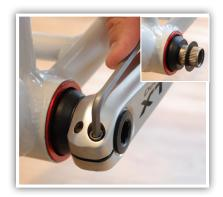
3. Install the crank. If there is side-to-side play, you may need 24 mm spacer(s) on the outside and/or additional 30 mm spacer(s) installed on the inside of the adapter. Tighten to manufacturer's specification. Crank should spin freely.
