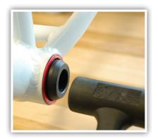
2. Insert the left side adapter. Spacers can be placed on either side to center cranks in bottom bracket.
