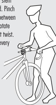
After installing the stem, check that the cable housings do not bind. Check by turning the handlebar until the grip hits the frame. If the housings bind, replace with longer ones.
