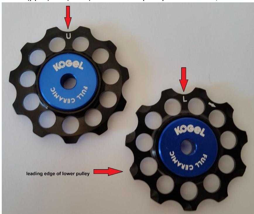
The pulley wheels are compatible with 11 speed drive trains for Shimano, Sram and Campagnolo. In the packaging you will find 4 washers to make the pulleys fit 10 speed Shimano and Sram. Install 1 washer on both sides of each pulley wheel.
