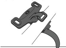
Feed the strap up and through the eyelet.
