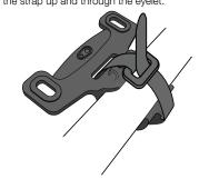
Pull the strap away from the bracket to apply tension.
