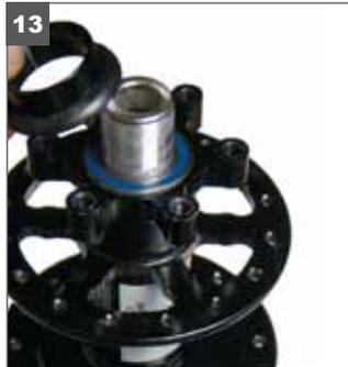
13. Grease the threads and install the spacer with dust seal. Hubs with serial numbers beginning with "D" or "E" or ending with "III" will not have this spacer.
