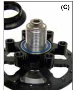
C. Remove spacer with dust seal. Hubs with serial numbers beginning with "D" or "E" or ending with "III" do not have this spacer.
