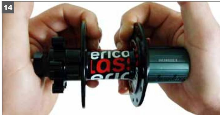
14. Holding the wheel by the hub flanges, use your palms to check if the axle moves side-to-side. If the axle moves side-to-side, tighten the lock and adjusting nuts slightly until it does not move side-to-side. When finished, the axle and cassette body should spin freely.
