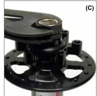
(C) Using two 19mm cone wrenches, remove all play on adjusting nut, then back off one half rotation, 180 degrees.
