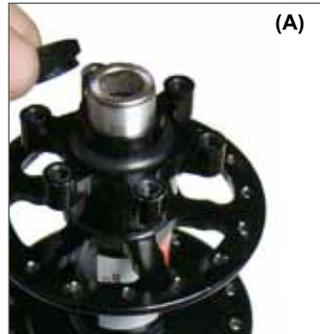
(A) Finger tighten the adjusting nut with the shoulder side facing the hub shell. For hubs with serial numbers beginning with "D" or "E" or ending with "III" install the dust seal on the adjusting nut.
