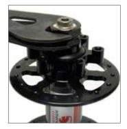
Using two 19mm cone wrenches, remove all play on adjusting nut, then back off one half rotation, 180 degrees. Holding the wheel by the hub flanges, use your palms to check if the axle moves sideto-side. If the axle moves side-to-side, tighten the lock and adjusting nuts slightly until it does not move side-to-side. When finished, the axle and cassette body should spin freely.
